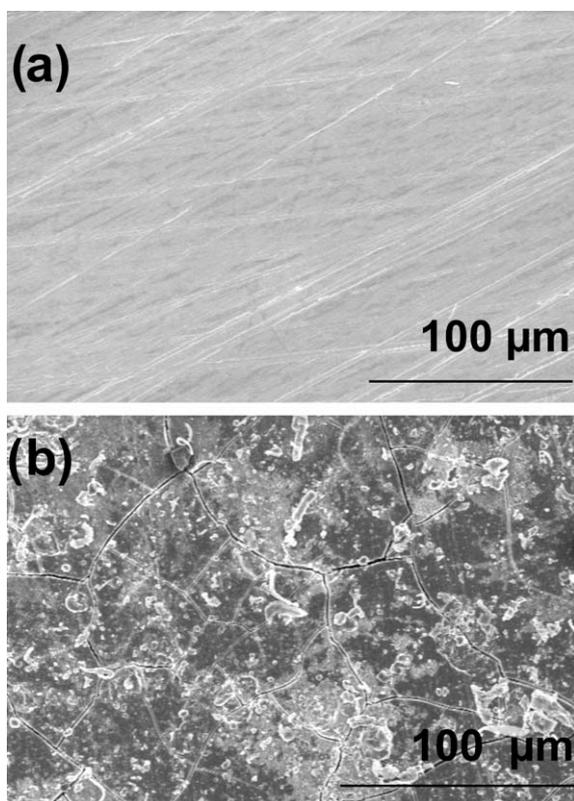
Fig. 1. SEM images of the surface of Mg samples soaked in: (a) 1 M NaOH for 24 h and (b) M SBF at 37 °C for 5 days.
