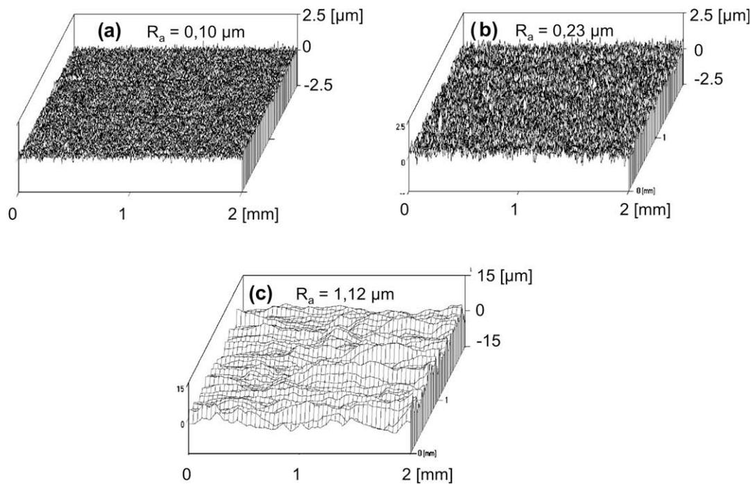
Fig. 2. Laser profilometry of the Mg surface: (a) polished; (b) soaked in 1 M NaOH for 24 h; and (c) soaked in M SBF at 37 °C for 5 days.
